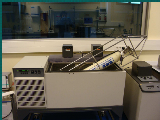
Photo 2 – CTD in the controlled temperature bath
